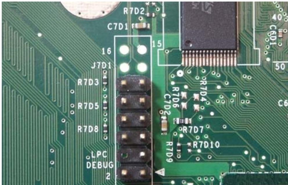
After reinserting the pin header, we will need to solder the pin header from the underside of the board, but before doing so you will need to temporarily secure the pin header or else it will fall out of the port when going to the underside of the board. Tape is a great way of going about doing it.
